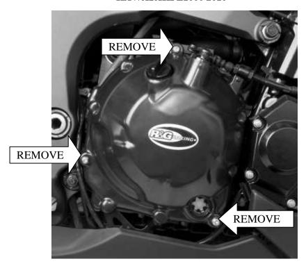
In this kit there should be: 1 x Engine Case Cover (ECC0079) 3 x M6x40mm long button head bolt
