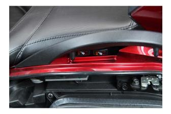
5. To operate heaters, use the switches located under the left handrail. The driver (front) heat is controlled by the forward switch, and the passenger (rear) heat is controlled by the rearward switch. For each switch: front = high heat, center = off, back = low heat.
