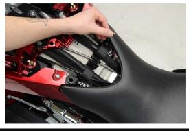
3. Lift the front of the seat up and carefully slide the seat forward out of the frame mount. Unplug the heater power connector located under the rear of the seat, then lift the seat up and forward to remove from the motorcycle. Note: Be extremely careful not to contact the fuel tank with the seat's front brackets.
