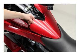
2. Using a 4mm Allen wrench, remove the two bolts at the front of the seat.
