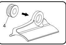
Install (No. 7) ALS-047 for Husqvarna OR ALS-056 for KTM, aluminum spacer in the backside of (No. 4) Z1023, rubber grommet and install (No. 5) ALS-046, aluminum spacer in the frontside as shown below.
