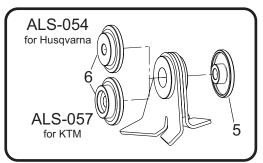
6. Install (No. 4) *Z1023,* rubber grommet into muffler bracket.
