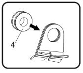
Install (No. 5) *ALS-046*, aluminum spacer in the front side of (No. 4) *Z1023*, rubber grommet and install (No. 6) *ALS-054 for Husqvarna OR ALS-057 for KTM*, aluminum spacer in the back side of (No. 4) *Z1023*, rubber grommet as shown below.
