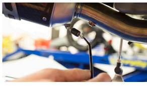
Reinstall O2 sensor onto TBR slip tube using supplied 12mm adapter kit and copper washer.
