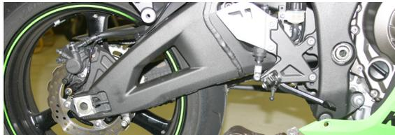
6. Remove lower right foot peg bolts and replace with supplied 8x35mm bolts.
