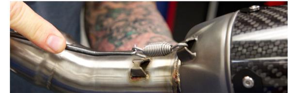
9. Slide supplied barrel clamp on end of slip tube where it will meet OEM head pipe. Fit loosely onto bike.
