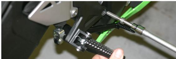
7. Install supplied mounting bracket as shown to the pre-installed supplied bolts, retain with supplied nuts.
