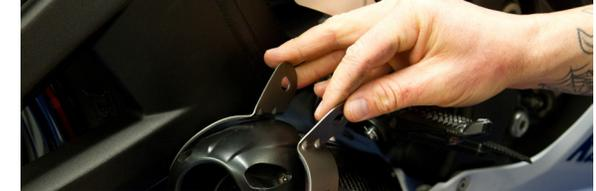
11. Loosely install muffler clamp to TBR bracket using the supplied 8x20mm bolt and nut.
