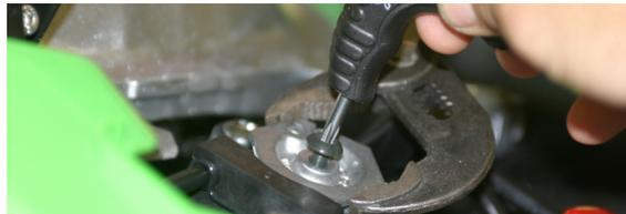
5. Remove OEM muffler assembly with servo cables.
