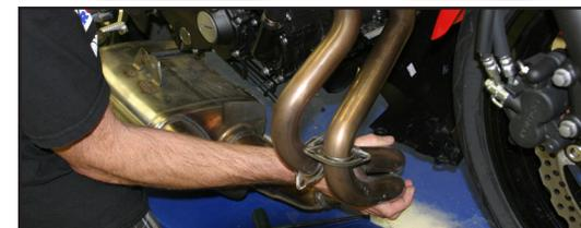
6. Attach supplied muffler mounting bracket to the three rubber mounting supports. Use supplied nuts and bolts.
