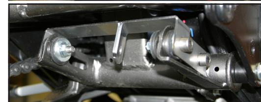
7. Loosely attach TBR muffler to TBR header using the supplied 6x20mm bolts, washers and X-ring.
