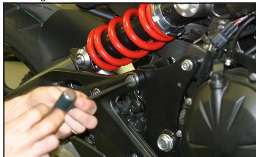
4. Remove muffler mounting hardware.
