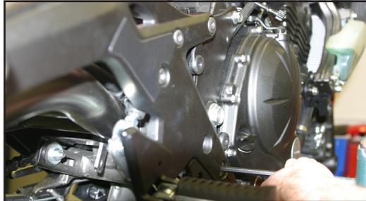
9. Slide the (rubber-lined) muffler clamp over the muffler canister and install header on bike using supplied flange bolt and nut on muffler clamp.
