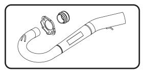
Install manifold and flange using the stock header nuts. Torque evenly to factory specifications.
