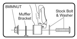
8. Torque muffler mount bolt to factory specification.
