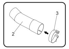
3. Install (No. 2) 11182-435D/11182-735D, tailpipe over the stock header outlet and align muffler bracket to the frontside of muffler mount as shown. Secure using the stock muffler mount bolt, washer, and nut. .
