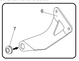
1b. Install (No. 7) *Z1022*, rubber bushing into (No. 18) *12651-MBKT*, muffler bracket.
