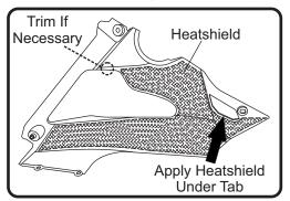
17a. Re-install right side lower cowl using the reverse steps of removal.
