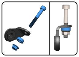
Install *ALS-043*, aluminum spacers into *b*ackside of Z1024, rubber grommet and ALS-059, aluminum spacer into frontside.
