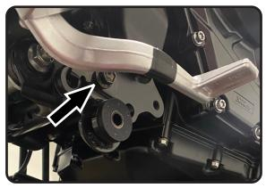
Remove right passenger footpeg pin by removing the E-Clip on the bottom and carefully remove footpeg pin.
