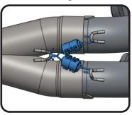
10. Install *RACE-SPX-2*, short springs between tailpipe to header connection and muffler to tailpipe connection.
