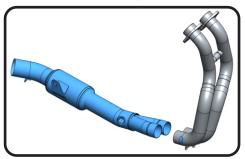
Install header and secure using stock header flange bolts and stock chassis mount bolt. Do not torque at this time.
