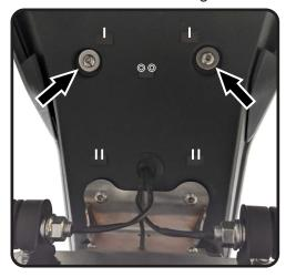
9. Install *16370-FEBKT-SPR*, fender eliminator clips to cover rectangle holes in undertail.
