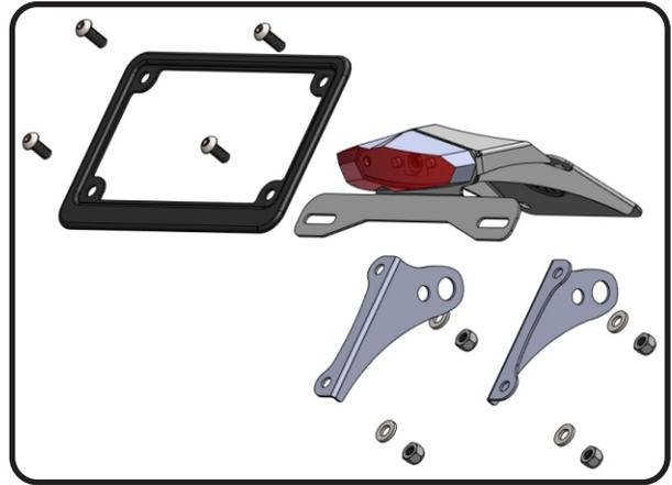
5. Install assembled fender eliminator by routing license plate light and turn signal wires through *H-2158*, wire cover on fender eliminator bracket and through undertail. Secure fender bracket to frame using the four stock fender bolts. Torque bolts to factory specification.
