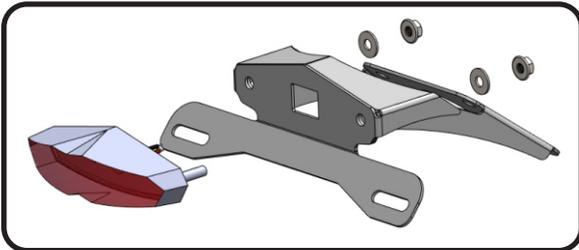
2. Install *H-2158*, wire cover into *11720-FEBKT*, fender bracket.
