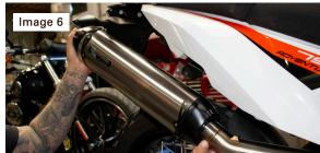
8. Slide supplied muffler clamp over your new S1R muffler. (Reference image 7)
