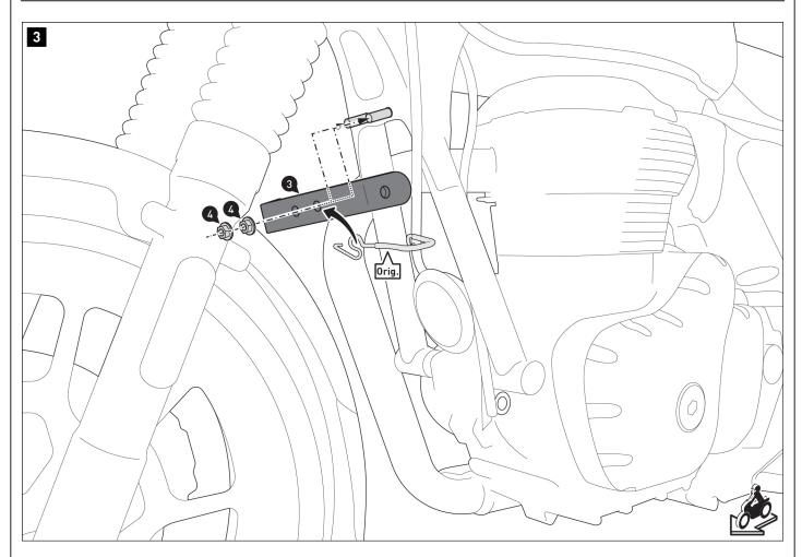
Screw the crossbar [3] to the original cable holder (Orig.) on the vehicle. **MOTE:** Make sure that the original cables are routed correctly again.
