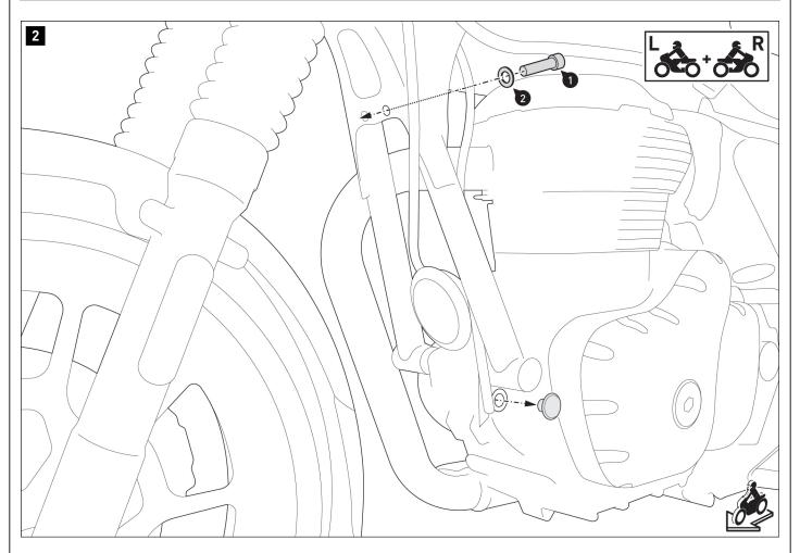
Insert the screw (1) with the washer (2) into the opening of the frame on both sides.
