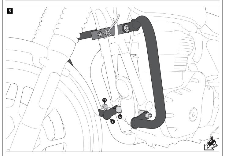
Screw the right half of the crash bar (6) to the screw (9) with the spacer (12) and the nut (13).
