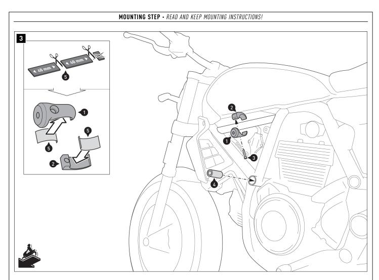
Cut the rubber strip (5) into two 40 mm pieces (the rest is no longer required). Then glue the rubber strips (5) into the clamps (1) and (2) as shown in the detailed drawing.
