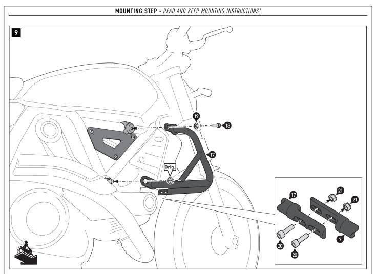
Install the right crash bar (17) on the vehicle. **A WARNING: Use a liquid threadlocker!** Do not tighten the screw (18) yet.
