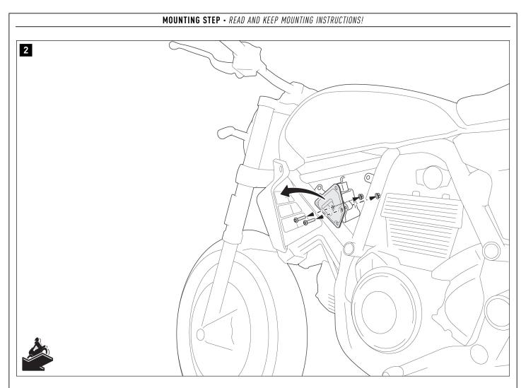
Remove the parts shown from the left side of the vehicle.
