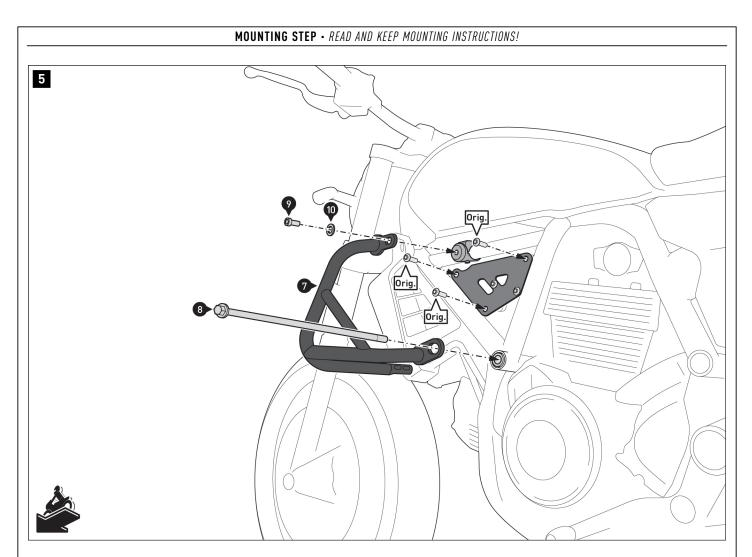
Mount the mounting bracket (6) with the original screws (Orig.) on the left side of the vehicle. **A WARNING: Use a liquid threadlocker!** Tighten the screws according to the manufacturer's instructions.
