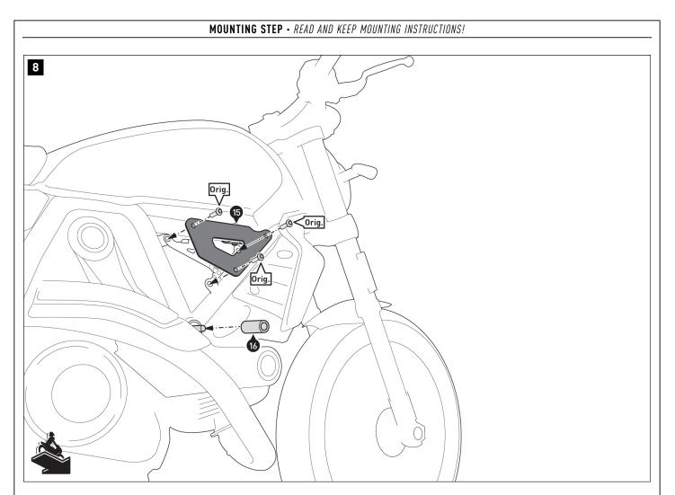
Mount the mounting bracket (15) with the original screws (Orig.) on the right side of the vehicle. **A WARNING: Use a liquid threadlocker!** Tighten the screws according to the manufacturer's instructions.
