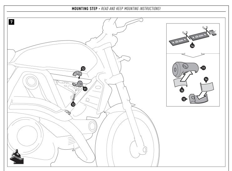
Cut the rubber strip (14) into two 40 mm pieces (the rest is no longer required). Then glue the rubber strips (14) into the clamps (11) and (12) as shown in the detailed drawing.
