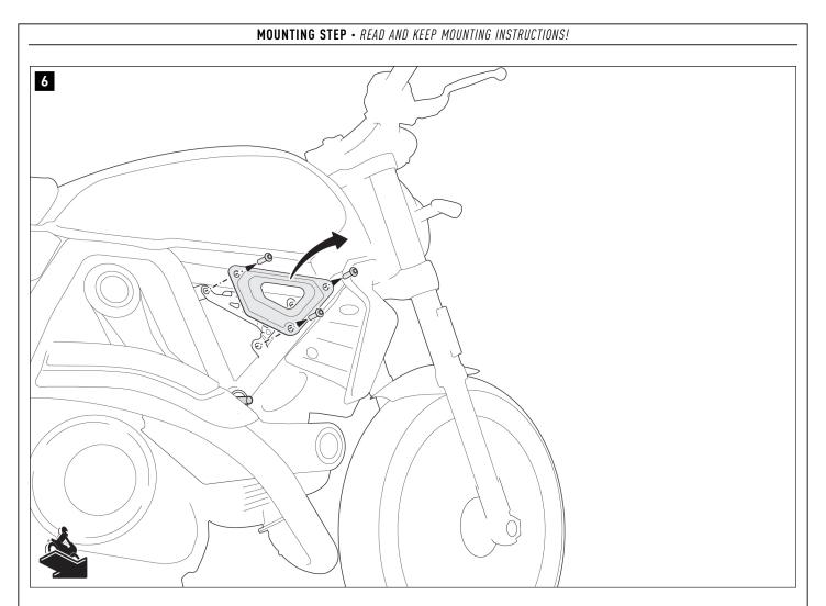
Remove the parts indicated from the vehicle.
