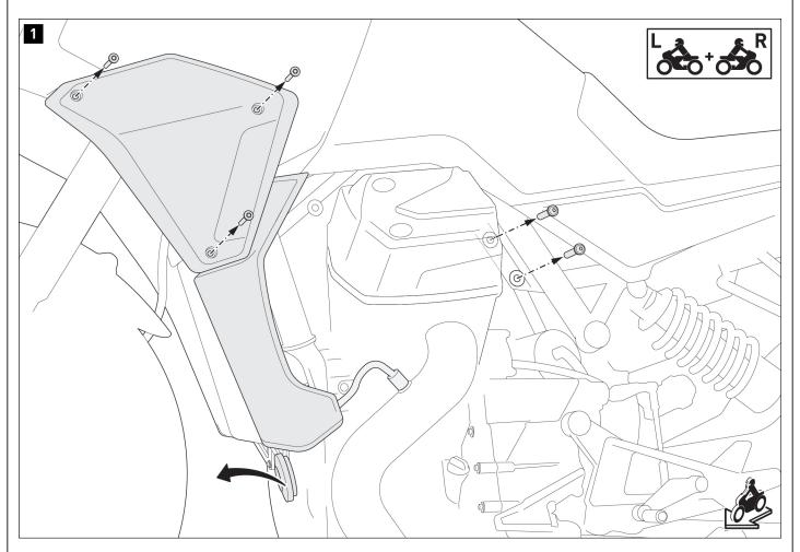
Remove the screws shown  ${\bf on\ both\ sides}$  and the top cover from the vehicle.
