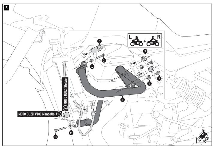
⚠ NOTE: The spacer (12) is for the MOTO GUZZI V100 Mandello on the left side. The spacer [13] is for the MOTO GUZZI V100 Mandello on the right side. The spacer [14] is for the MOTO GUZZI Stelvio on the left side. The spacer [15] is for the MOTO GUZZI Stelvio on the right side.
