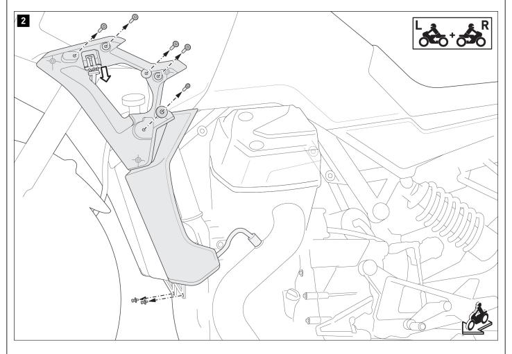
Disconnect the plug connections of the inner fairings on **both sides**. Remove the original screws and washers. Remove the interior fairing s from the vehicle.
