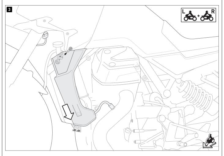
Remove the original screws and the lower fairing s from the vehicle **on both sides**.
