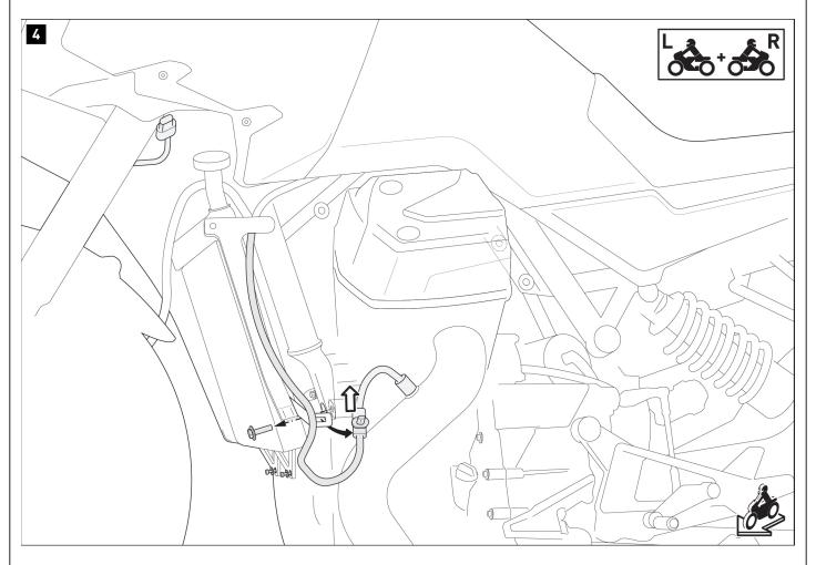
Remove the original screws **on both sides** of the vehicle.
