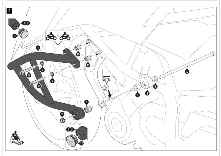
Insert the plastic plugs (3) into the openings of the crash bar (1/2).
