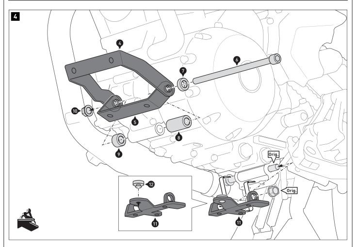
Screw the front mounting brackets (4) (outer) and (5) (inner) to the vehicle. Roughly position mounting brackets (4) and (5) as specified in the illustration. Do not tighten the screw (6) yet.
