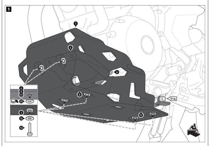
Use some grease to attach the washers (15) to mounting brackets (4), (5) and (11).
