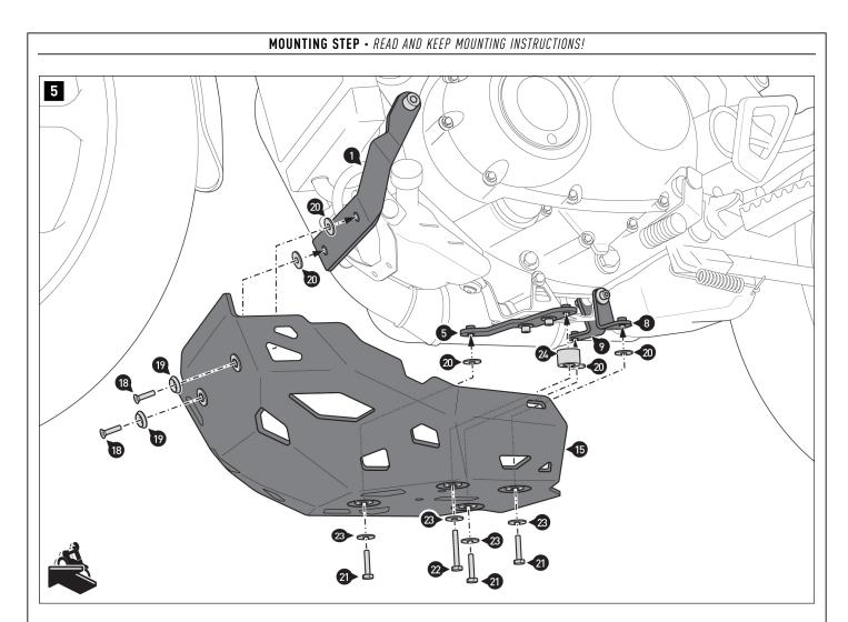
$\triangle$  NOTE: Use some grease to stick the washers (20) to the mounting brackets.
