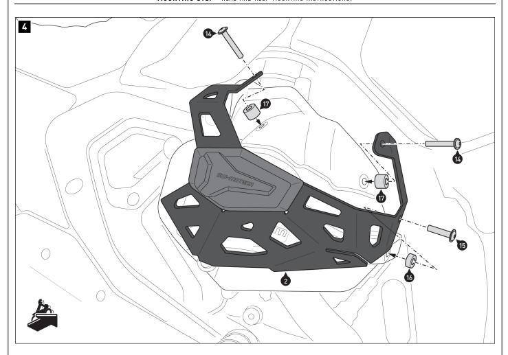
Screw the mounting bracket (2) onto the **right** cylinder. **A WARNING:** Use a liquid threadlocker!
