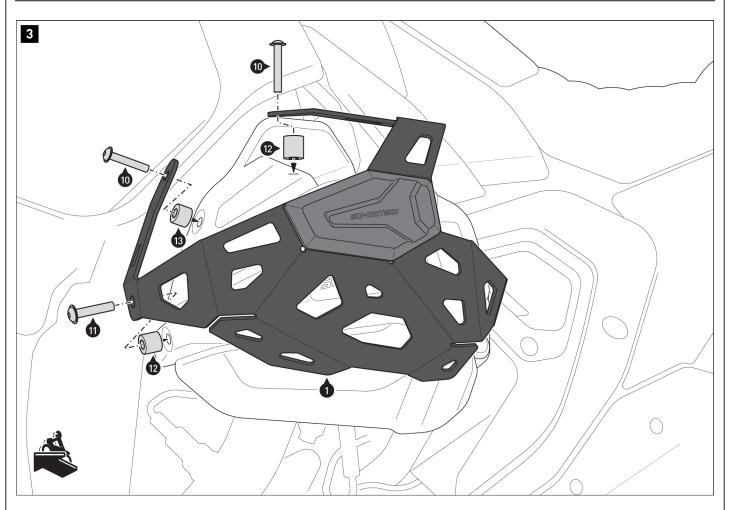
Screw the mounting bracket (1) onto the **left** cylinder. **A** WARNING: Use a liquid threadlocker!
