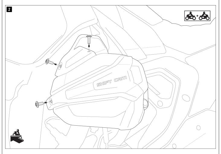
Undo the screws indicated on  ${\bf both\ sides}$  of the cylinder panelling.
