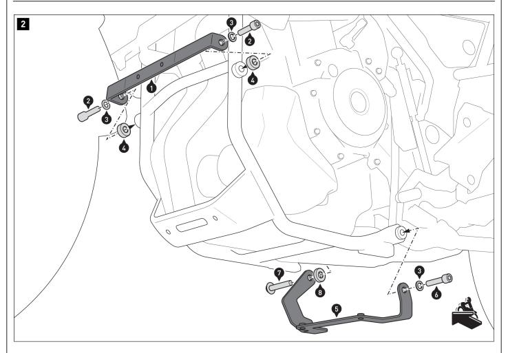
$\triangle$  **NOTE:** The spacers (4) are not required in conjunction with the SW-MOTECH crash bar. In their place, mount the crash bar with the parts of the engine guard.
