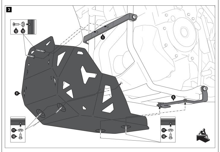
Screw the engine guard [9] to the mounting brackets (1) and (5).  $\triangle$  WARNING: Use a liquid threadlocker!
