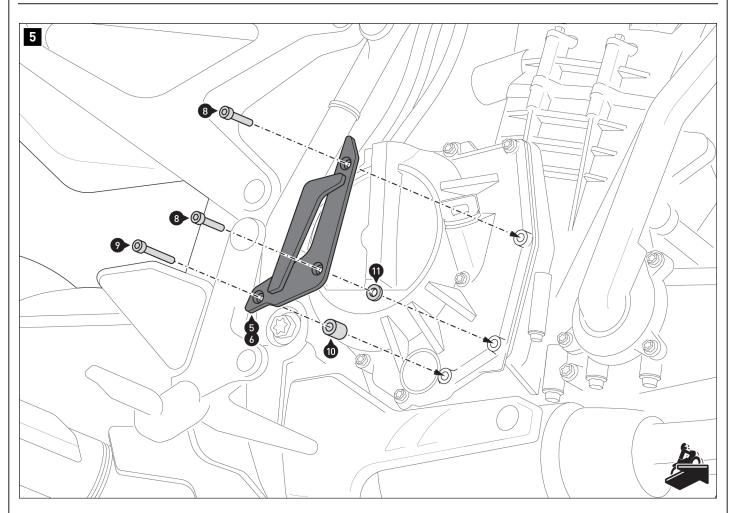
Screw the parts [5/6] onto the vehicle.
