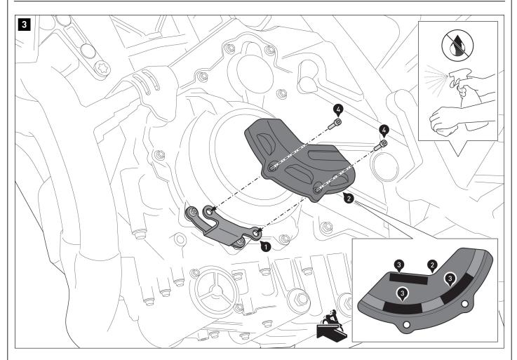
Glue the protective strips [3] to the back of the alternator cover protector [2] as shown in the detailed drawing.
