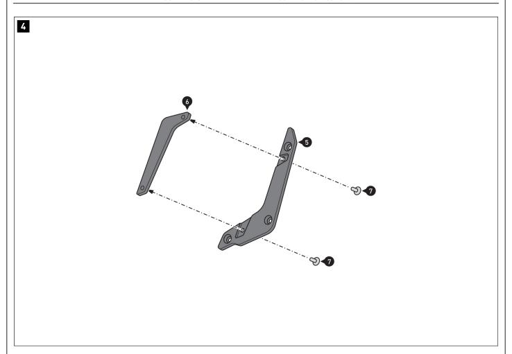
Screw the milled part [5] to the outer milled part (6).
