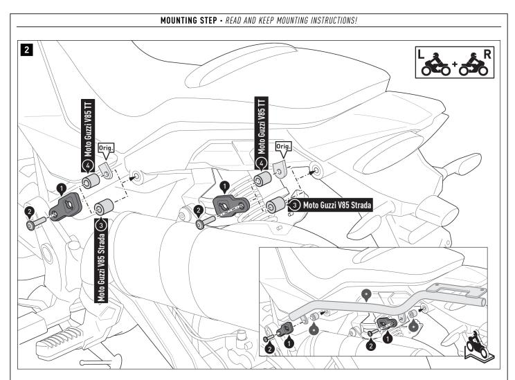
$\triangle$  **NOTE:** The parts of the OEM luggage rack (Orig.) of the vehicle model V85 TT shown are schematic and are intended only as a guide during installation.
