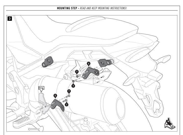
Attach the mounting bracket (5) with the original heat shield (Orig.) ( **left side of the vehicle** ) and the fastening tab (6) (**right side of the vehicle** ) on the vehicle.
