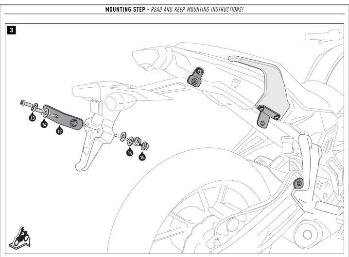
Screw the crossbar (12) to the license plate holder. Do not tighten the screws yet.
