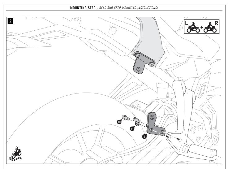
Screw the mounting brackets (8) and (9) on both sides of the vehicle behind the passenger footrests. **A WARNING: Use liquid threadlocker!** Do not tighten the screws yet.
