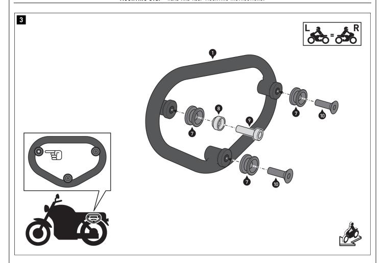
Screw parts (7) to (10) onto the side carrier (1).
