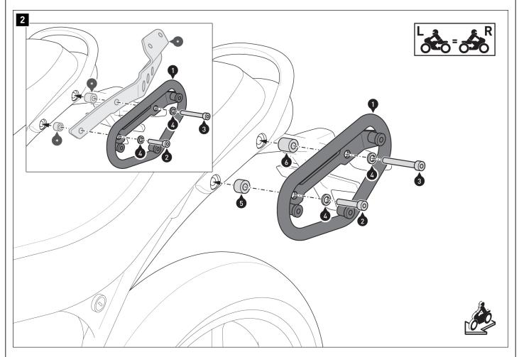
⚠ NOTE: If you are installing the luggage rack at the same time as the SW-MOTECH luggage rack (\*), screw the parts together as shown in the detailed drawing. Spacers (5) and (6) are not required. Instead, install the spacers (\*) included with the luggage rack.
