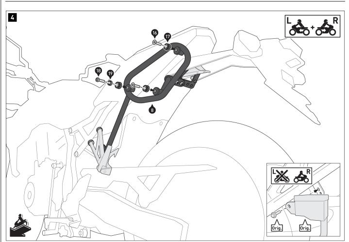
Screw parts [16] to [19] to the side carrier [8] and [9]. **A WARNING: Use liquid threadlocker!** Tighten screws [16] and [18] as specified in the instructions.
