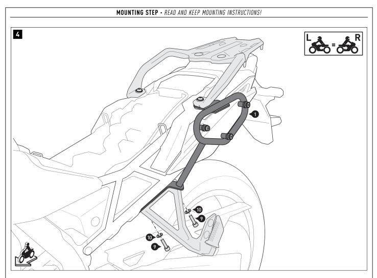
Screw the side support (1) to the footrest on the vehicle. **A** WARNING: Use liquid threadlocker! Now tighten the screws (6) and (9) according to the manufacturer's instructions.
