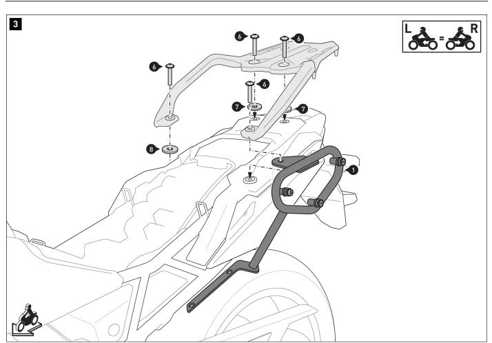
Screw the side carrier [1] to the original luggage rack on the vehicle. **A WARNING: Use a liquid threadlocker!** Do not tighten the screws yet.
