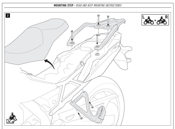
Remove the seat from the vehicle according to the vehicle manual.
