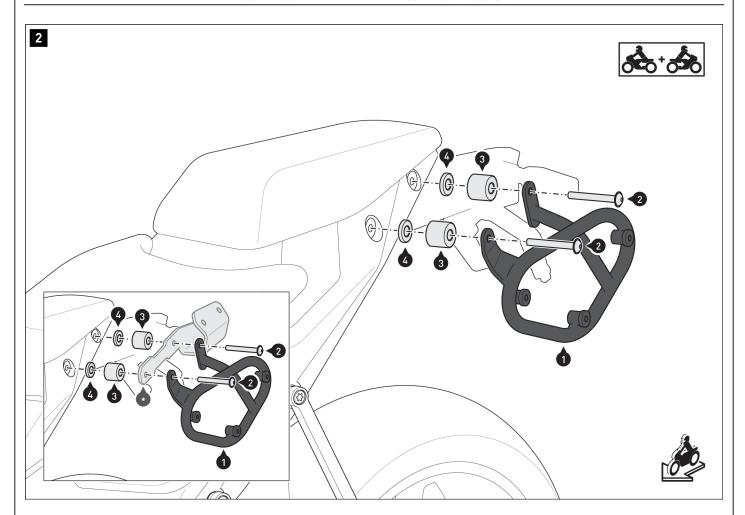
$\triangle$  **NOTE:** If the side carrier (1) is to be mounted together with the SW-MOTECH rack, screw the rack mounting bracket (\*) as illustrated in the detailed drawing.
