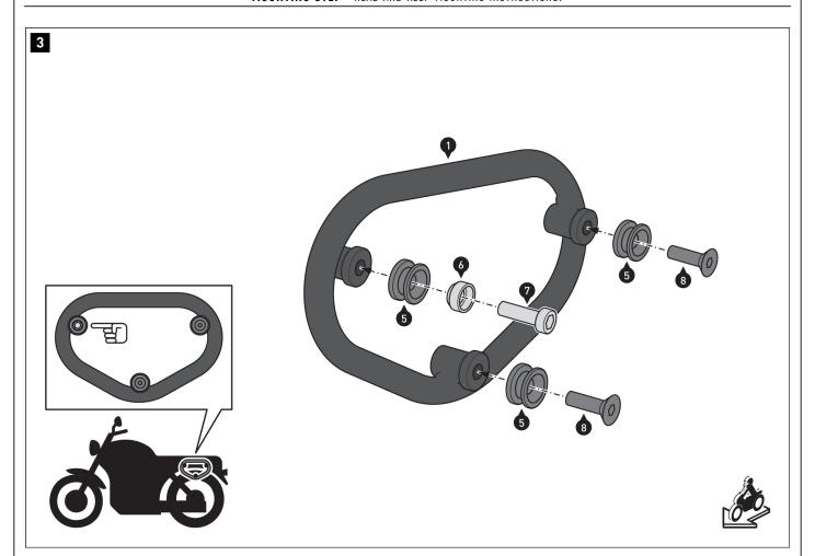
Screw parts (5) to (8) to the side carrier (1). **A** WARNING: Use a liquid threadlocker!
