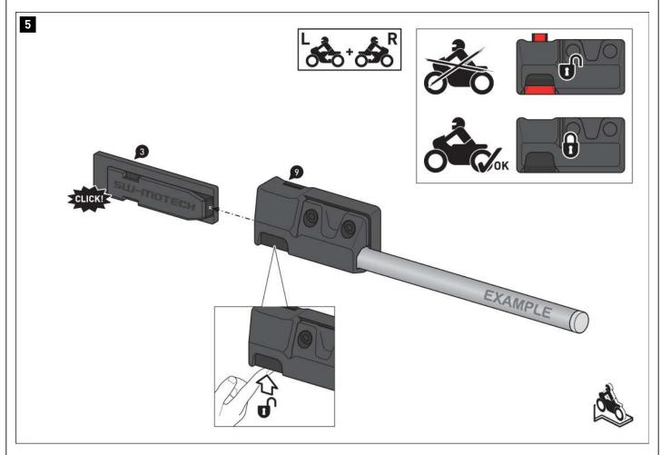
Slide the plug connectors (9/10) onto the connector mounting rails (3/4) on both sides.
