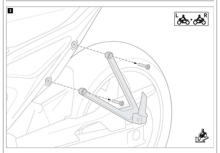
Remove the original parts shown here from the vehicle.
