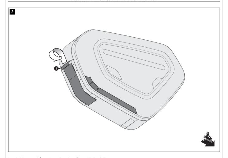
Loop the Velcro strap (1) onto the rear loop of your Blaze saddlebag. Pull the Velcro strap (1) until taut.
