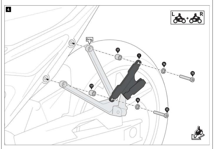
Screw the mounting brackets [1/2] onto the vehicle.
