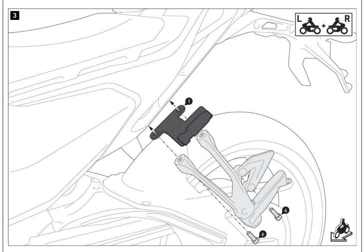
Screw the mounting brackets (1/2) to the passenger footrest bracket on the vehicle.
