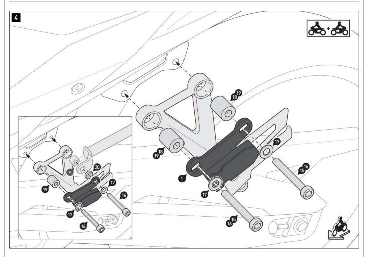
$\triangle$  NOTE: HONDA CB500X (13 –), CBR300R (15 –), NX500 (24 –): Install the mounting brackets (1/2) on both sides with the screws (15) and the spacers (18).
