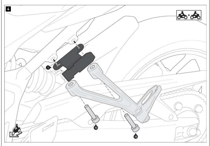
Screw the mounting brackets [1/2] to the passenger footrest holders on the
