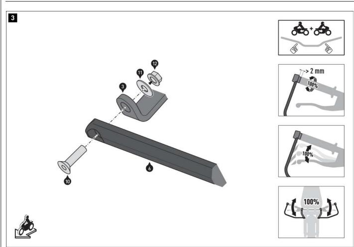
Screw the inner ends of the brackets (6/7) to the connecting plates (3/4). Do not tighten the screws (10) yet.
