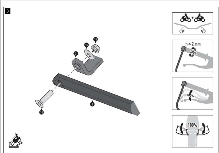
Screw the inner ends of the brackets (6/7) to the connecting plates (3/4). Do not tighten the screws (14) yet.
