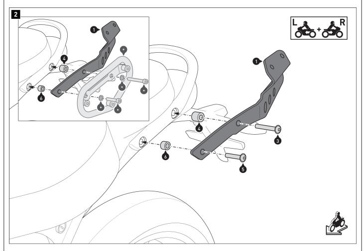
$\triangle$  **NOTE:** If installing at the same time as the SW-MOTECH side carrier (\*), screw the parts together as shown in the detailed drawing. Screws (3) and (5) are not required. Instead, mount the washers (\*) and screws (\*) included with the side carrier.
