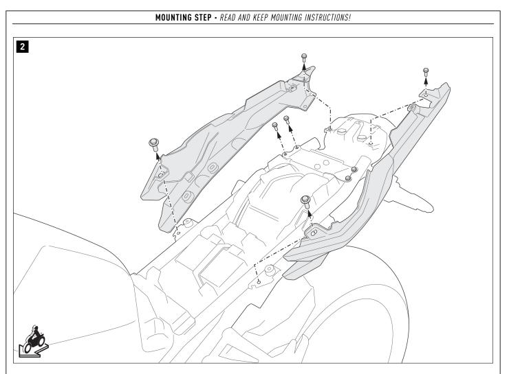
▲ **NOTE:** First remove the screws of the seat lock holder on one side only! Only remove the screws on the opposite side when the first side arm is already loosely screwed in.
