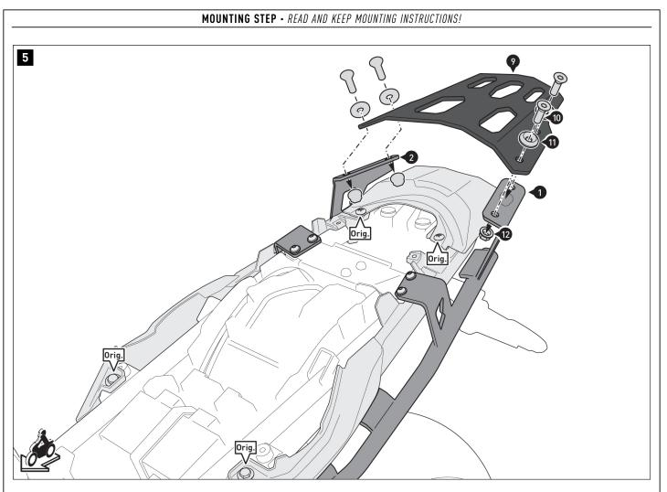
Screw the rack (9) onto the mounting struts (1) and (2).
