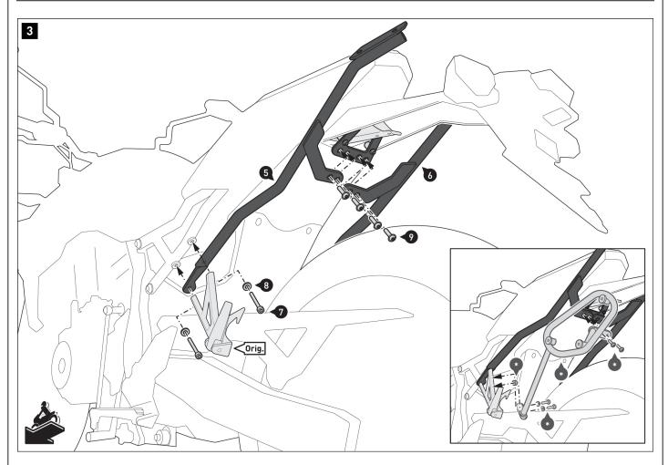
$\triangle$  **NOTE:** If the SW-MOTECH side carrier is mounted at the same time, the screws (9) are omitted. In their place, mount the screws (\*) included with the side carrier as shown in the detailed drawing.
