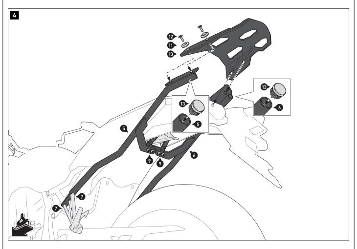
Insert the plastic plugs (13) into the ends of the mounting struts (5) and (6).
