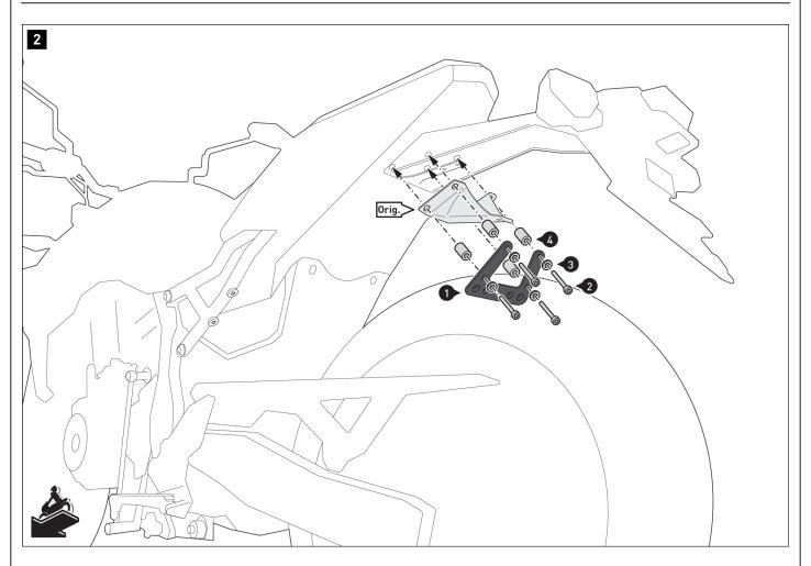
Screw the carrier plate (1) to the original cover (Orig.) and the parts shown at the rear of the vehicle.
