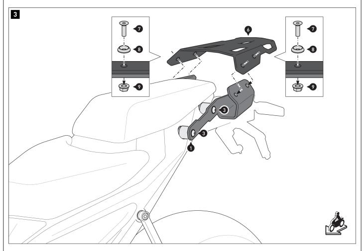
Mount the luggage rack (6) on the mounting bracket (1/2). **A** WARNING: Use a liquid threadlocker!
