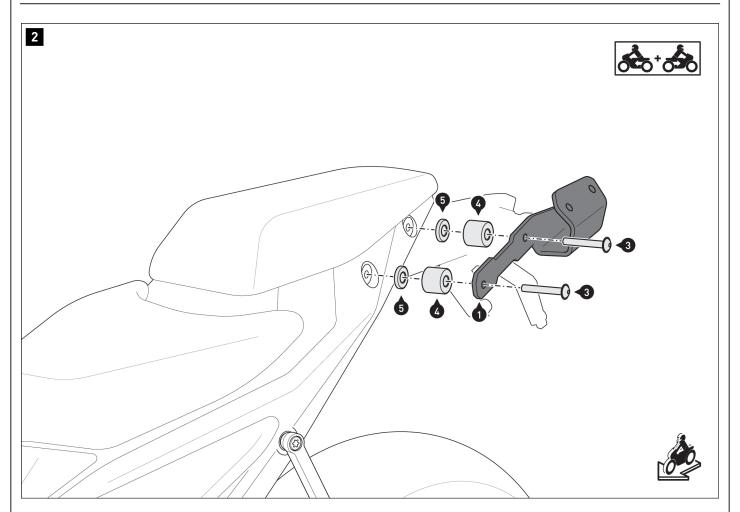
Mount the mounting brackets (1/2) on the vehicle. **A** WARNING: Use a liquid threadlocker!
