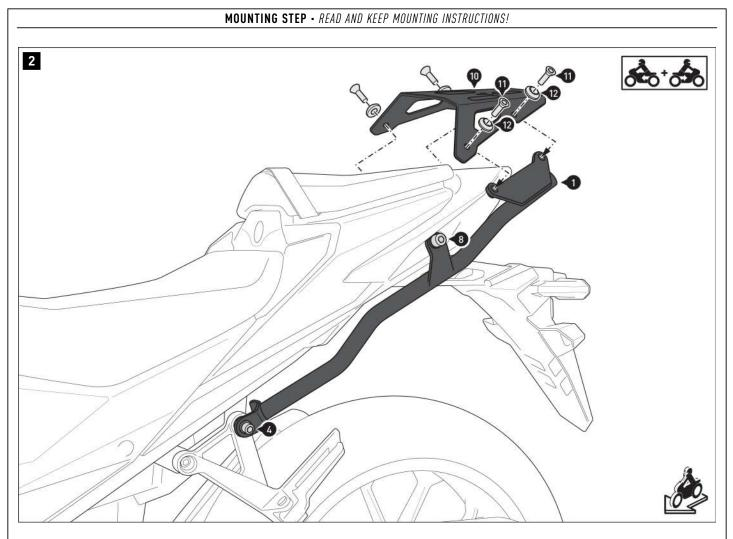
Screw the rack (1) onto the mounting struts (1/2). **A** WARNING: Use a liquid threadlocker!
