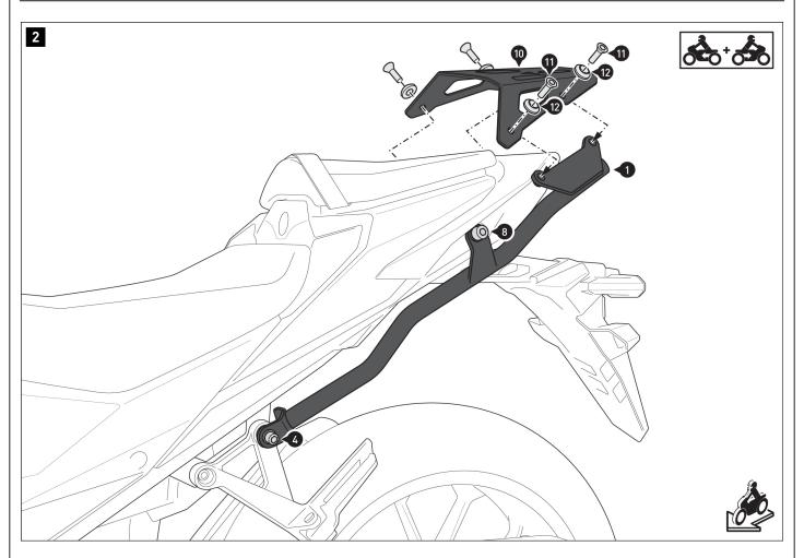
Screw the rack [1] onto the mounting struts [1/2]. **A WARNING:** Use a liquid threadlocker!
