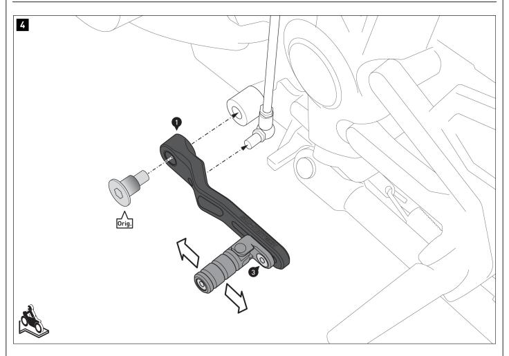
Coat the original screw (Orig.) with grease.
