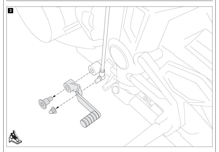
Loosen the bolt and nut and remove the original gear lever from the vehicle.
