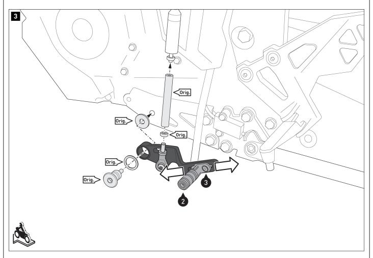
Screw the original deflection rod (Orig.) to the gear lever (1) (min. 6 threads); lock the thread with the two original nuts (Orig).
