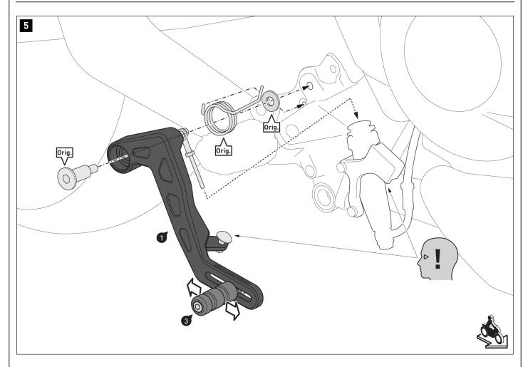
Screw the brake lever (1) to the vehicle using the original parts (Orig.).
