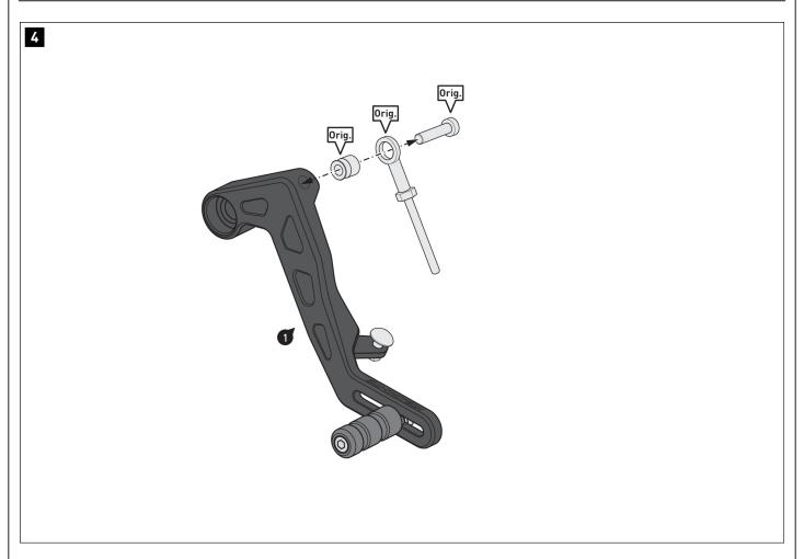
Screw the original parts (Orig.) shown to the gear lever (1). **A** WARNING: use liquid thread locker!
