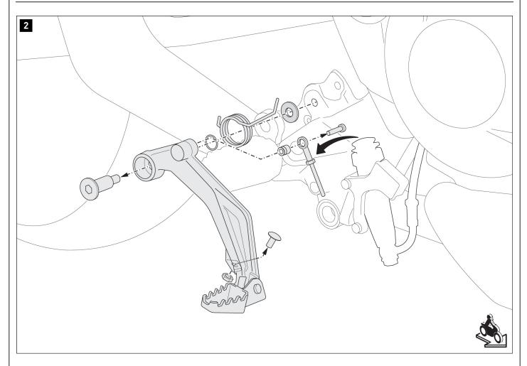
Loosen the screws indicated and remove the original gear lever from the vehicle.
