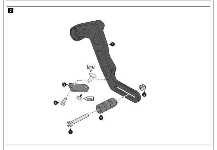
Screw the parts indicated as well as the original parts (Orig.) to the gear lever (1).
