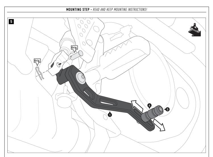
Connect the brake pedal (1) to the brake master cylinder. Use the original parts (Orig.). Adjust the pedal (4) according to your driving habits; then tighten the screw (5) as specified in the mounting instructions.
