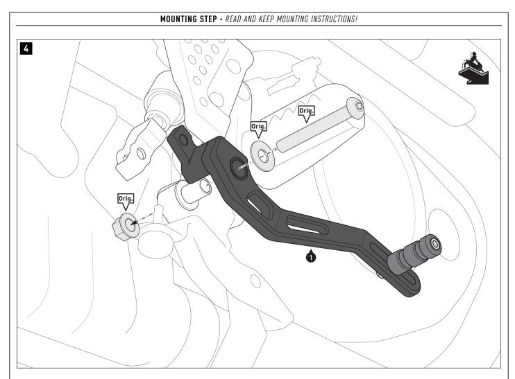
Screw the brake lever (1) to the vehicle using the original parts (Orig.). Tighten the original screw (Orig.) according to the manufacturer's instructions.
