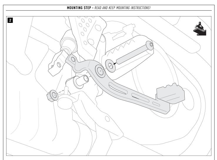
Remove the original brake pedal and the parts shown from the footrest mount.
