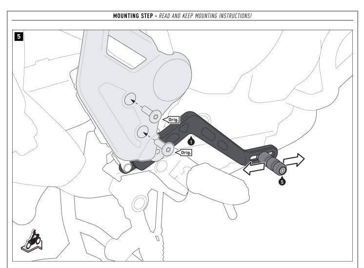
Adjust the pedal (4) according to your driving habits; then tighten the screw (5) as specified in the mounting instructions.
