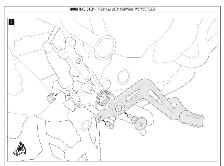
Unscrew the lock washer and bolt from the master cylinder.
