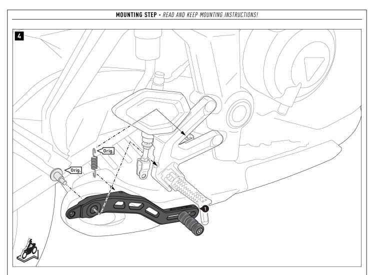
Screw on the brake pedal (1) behind the footrest using the original parts (Orig.). A WARNING: Make sure you insert the ends of the original spring (Orig.) in the holes provided! A WARNING: Use a liquid threadlocker! Tighten the original screw (Orig.) according to the manufacturer's instructions.
