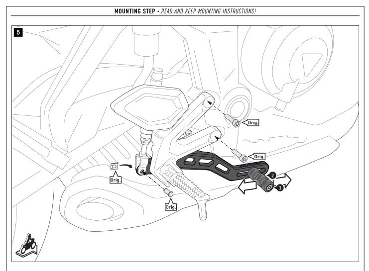
Finally, screw the footrest back onto the vehicle. **A WARNING: Use a liquid threadlocker!** Tighten the original (Orig.) screws according to the manufacturer's instructions.
