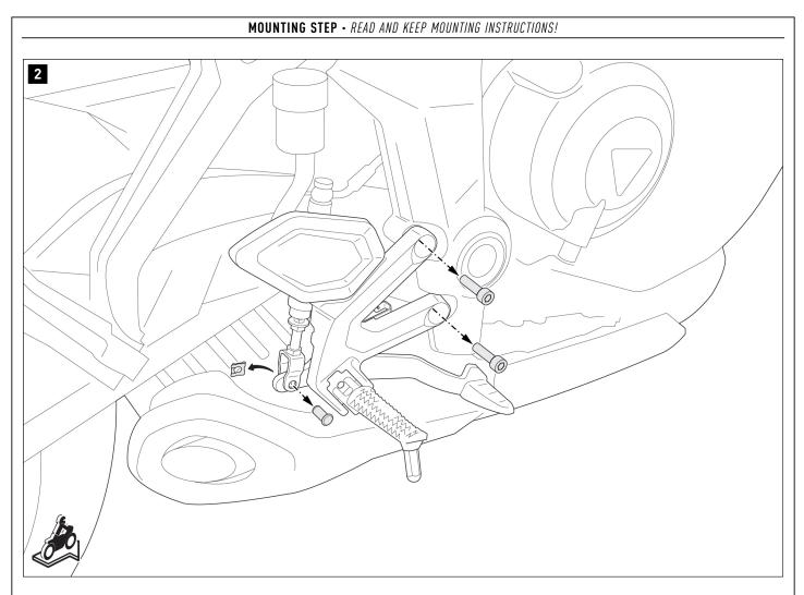
**NOTE:** Before disassembling the original brake pedal, note the order and orientation of the original parts.
