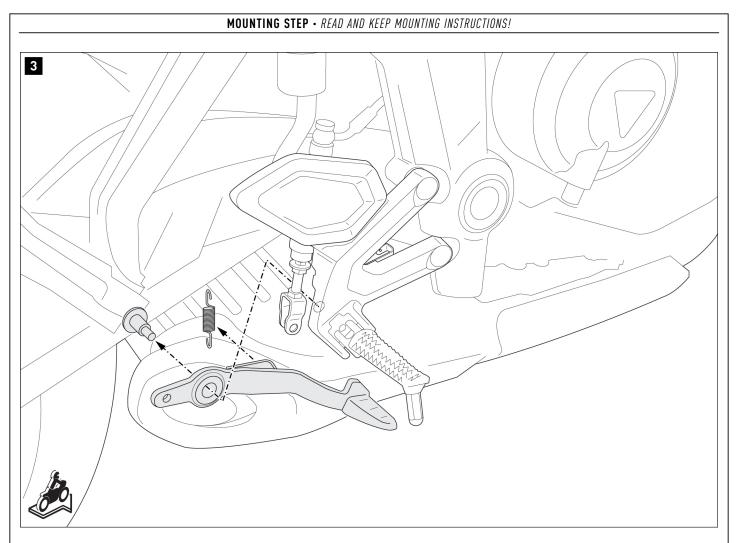
Loosen the indicated screws and unhook the spring.
