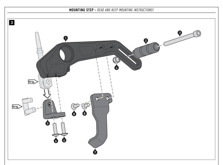
Screw the parts shown together. A WARNING: Use liquid thread locker (screws (6) and (8))! Do not tighten the screw (3) yet. Tighten the screws (6) and (8) as specified in the mounting instructions.
