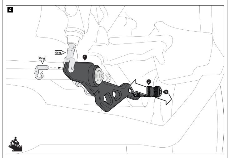
Secure the pressure bar using the original locking clip (Orig.).
