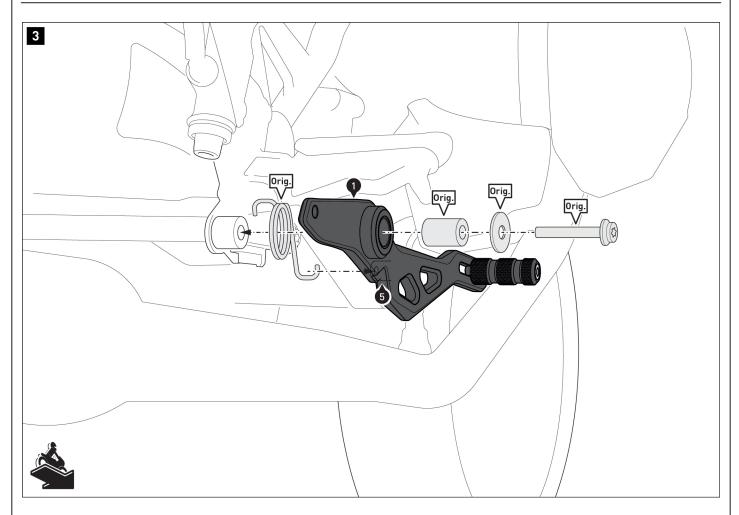
Screw the brake pedal (1) to the footrest system using the original parts (Orig.).
